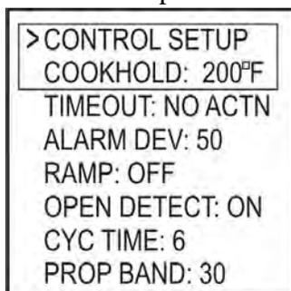
Scroll through values in the CONTROL SETUP SCREEN using the UP/DOWN keys. To modify a value press the M/E key. Use the LEFT/RIGHT keys select the digit to be modified. Adjust the value with the UP/DOWN Keys. Press the M/E key to save. To return to the MAIN SREEN press the UP and DOWN keys together.
