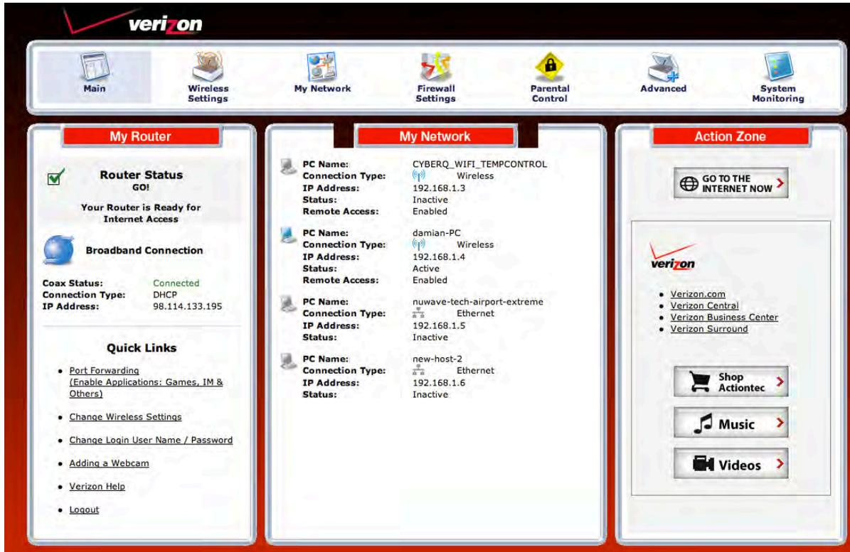
Create a new port forwarding rule by selecting CYBERQ\_WIFI\_TEMPCONTROL under the "Specify IP" dropdown and select "HTTP" under the application dropdown. Then click Add and then click Refresh and it should now appear in the list. Note that the CyberQ Wifi's IP address (192.168.1.3) was assigned to port 80. 80 is the default port number used by all web browsers to get web pages using HTTP (Hypertext Transfer Protocol).
