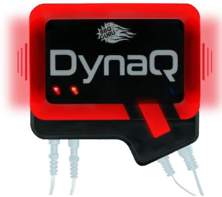
If the pit temperature is within its strategy range and the fan is blowing, the top and bottom of the outer Q ring will remain solid red while the left and right sides pulse red.
