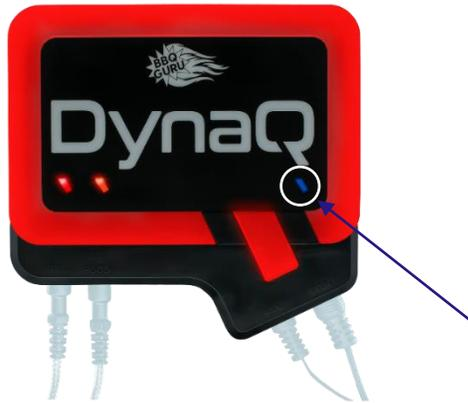
When the DynaQ is not connected to another device, the blue connectivity LED indicator light will blink slowly.
