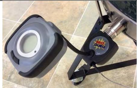
**Step 3** – Clip the pit probe to the top of the cooking grate inside your cooker and turn the power switch on. Adjust the setpoint using the UP ▲ DOWN ▼ keys.
