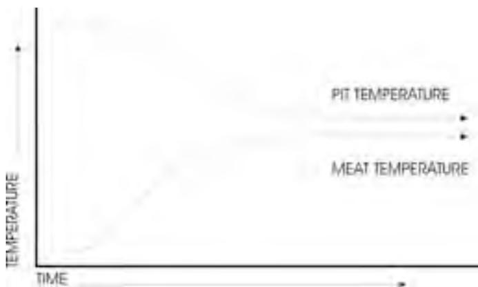
The BBQ GURU's Low-and-Slow Ramp Mode cooking response – This graph shows a higher than normal starting temperature being used. When in Ramp Mode The BBQ GURU allows a faster heat up of the meat without overshooting the desired internal meat temperature.
